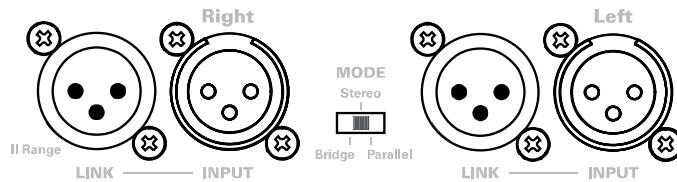
Between the input signal connections of the both channels is an operational mode switch provided. By means of this switch, the operational mode of the amplifier can be selected. There are three different operational modes available:
