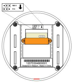
In most cases, the speaker cable will be provided through the wall, making the cable completely invisible from outer side. In some cases, the cable should be fed from outer side. For this purpose, a spot (marked in RED) with thinner material is provided at the bottom side, which can be removed using a plier for feeding the cable into the circular bracket.
